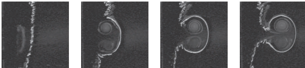
Fig. 2. Dye visualization of a dipole propagating through a line of dye. The dye eventually demarcates the interior region of the dipole which provides an indication of the separatrix aspect ratio.
